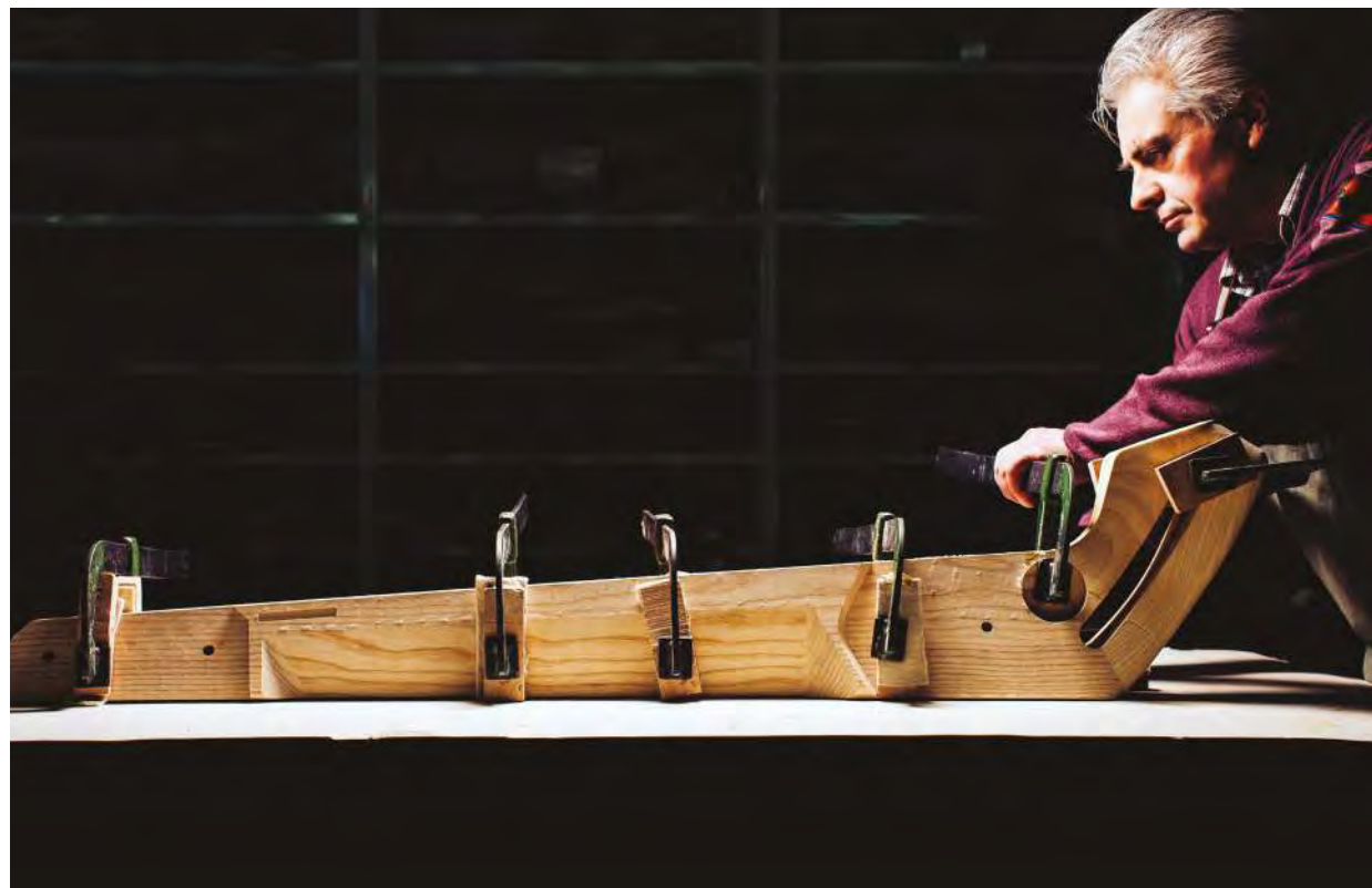
Accurate, numerically-controlled three-axis milling cutters carve the solid wood, later finished by the experienced craftsman.
